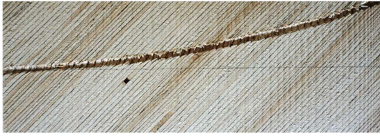
Figure 6: Deviation of a screw 8x320 in LVL at \alpha = 45^\circ .
