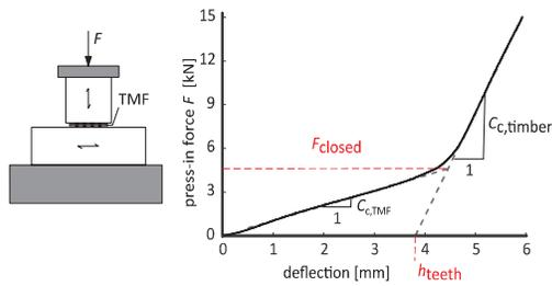
Figure 4: Penetration tests with samples of TMF dimensions 50x50 mm
