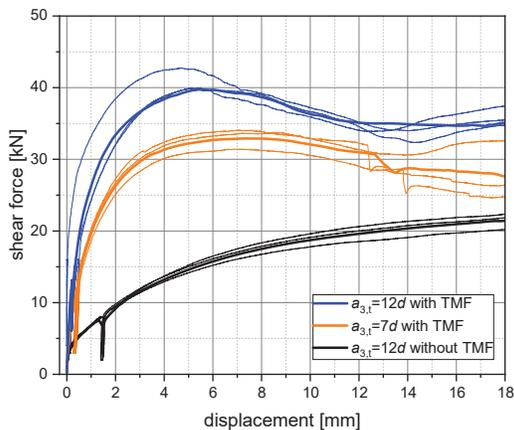
Figure 13: Results of shear tests with varying distances to the loaded end grain  $a_{3,t}=12 \cdot d$  and  $7 \cdot d$  with and without TMF reinforcement
