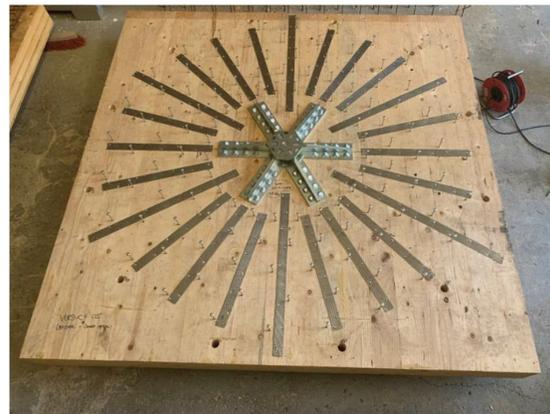
Figure 20: Preparation of the punching specimen with Spider Connector [16] and radial arranged TMF strips on the top surface
