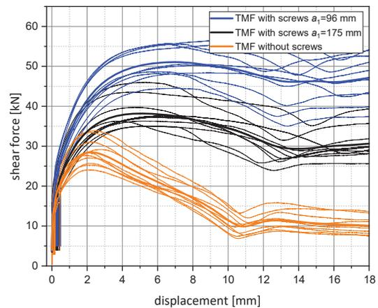
Figure 9: Load-deformation graphs: Shear tests with a length of 500 mm, with and without screws and varying amounts of screws
