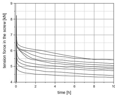
Figure 6: Tensile forces in a screw after screwing in, relaxation over a time period of 10 h
