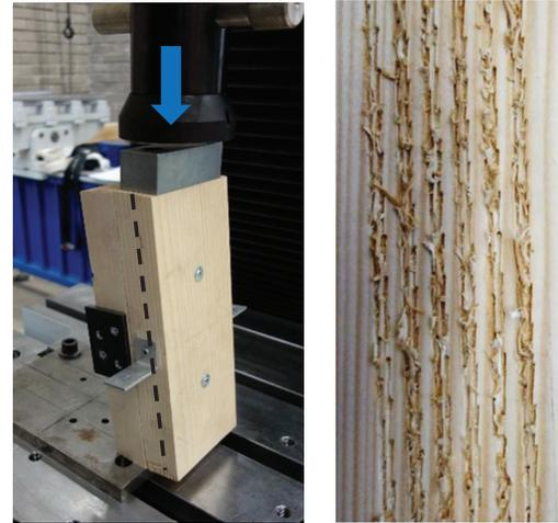
Figure 8: Preliminary inclined-shear tests: Comparison with single screw connection and TMF reinforcement and failure mechanism TMF
