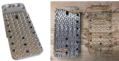
Figure 17: The modified surface of a joist hanger and failure mechanism after reaching the maximum load
