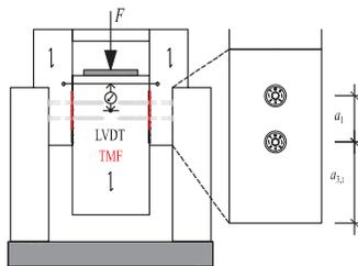
Figure 12: Shear tests with reduced minimum screw distances to the loaded end grain,  $a_{3,t}$  (modified test setup for preliminary tests [10])
