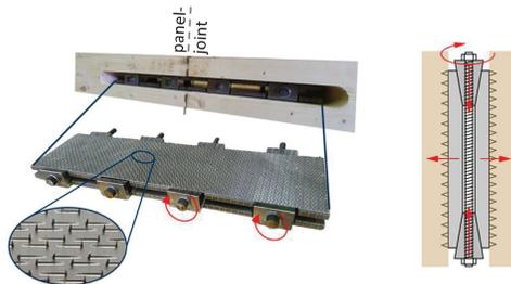
Figure 19: CLT edge connection with thicker metal plates and serrated surfaces
