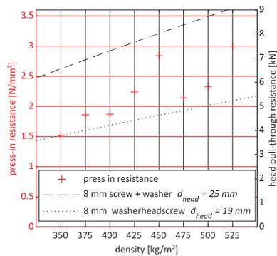
Figure 5: Influence of the gross density on the penetration (compressive) stresses in the side grain of softwood
