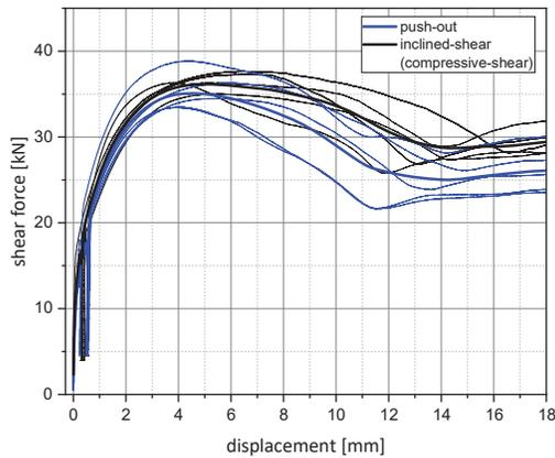
Figure 11: Load-deformation graph of different test methods: Inclined-shear and push-out tests (one and two-shear planes)
