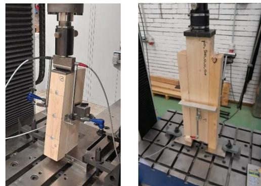
Figure 10: Different test methods: Inclined-shear (compressive-shear, left) and push-out tests (right)
