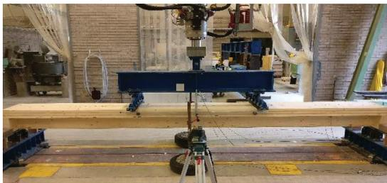
Figure 14: Bending tests with ribbed panels, span 6 m
