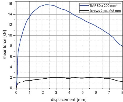
Figure 7: Load-deformation graphs: Comparison with a single screw connection and the TMF, preliminary tests
