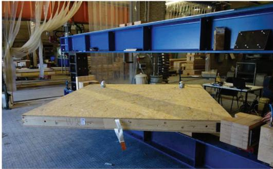
Figure 16: Diagonal test setup to determine the shear stiffness
