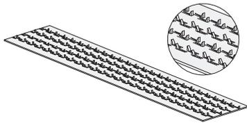
Figure 2: Toothed metal fastener (TMF) with scratched-out teeth on both sides
