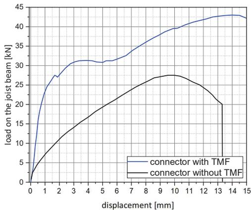
Figure 18: Shear tests of joist hangers with (blue graph) and without (black graph) TMF technology
