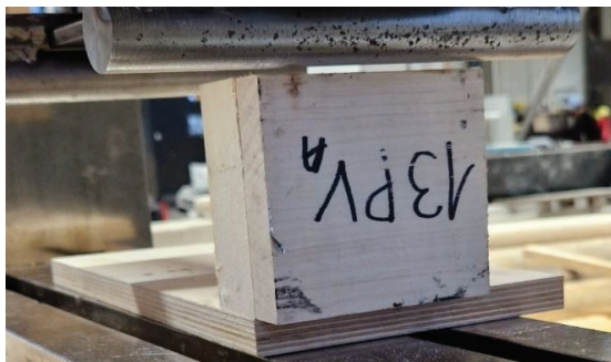
Figure 1. Test specimen tested at 20°C for shear capacity. Specimen is attached to a horizontal auxiliary board to avoid movement during the test and allow deformations. On top of the lamella closest to the camera the testing machine can be seen, which applies force to the lamella.
