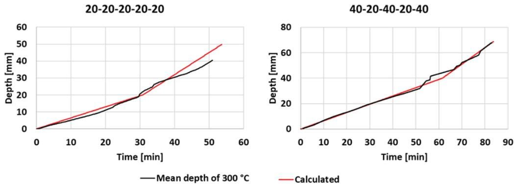
Figure 5. Measured mean depth of 300 °C isotherm (char depth), and calculated charring depth using the stepped charring model.
