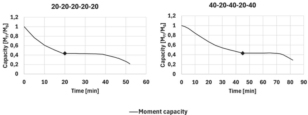
Figure 6. Tested panels' loadbearing capacity. The diamond represents the point where stresses in the lowest lamella exceed its strength before the cross-section reaches its highest capacity.
