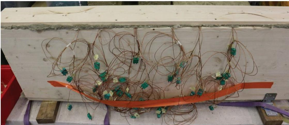
Figure 1. Overview of a test specimen showing the thermocouple wires drilled from the side face of the specimen and fire protection measures to limit heat flow and prevent excessive charring near the specimen corners.
