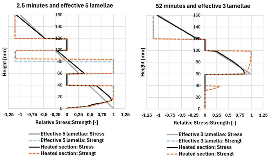
Figure 4. Stresses and timber strength in 40-20-40-20-40 panel cross section. The compression strength and tensile strength ratio is  $f_c/f_t = 0.9$ .
