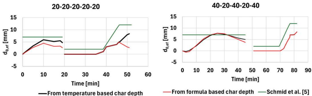
Figure 7. Effective ZSL in panels during standard fire.
