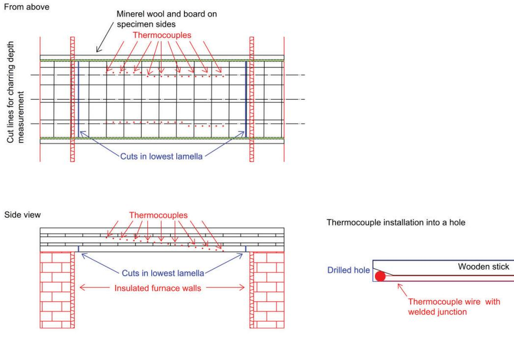
Figure 2. Schematic views of the test furnace, the specimen and the positioning of thermocouples: (a) plan and (b) vertical side views of the specimen, and (c) a thermocouple installation into a hole.
