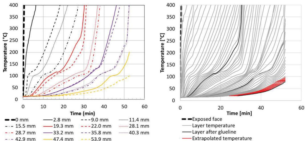
Figure 3: Left side is temperatures measured from one 20-20-20-20 station. The right side is interpolated temperatures middle of 1 mm layers.
