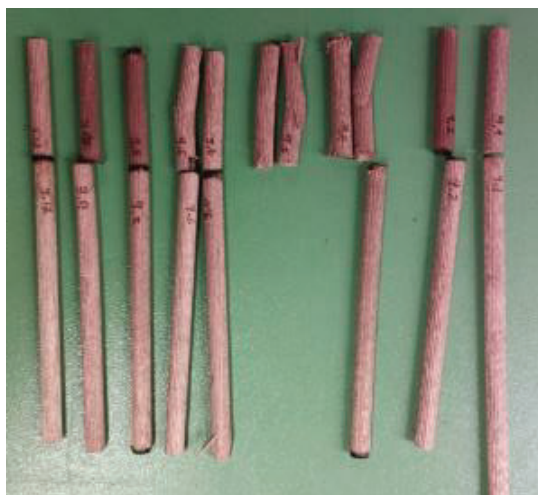
Figure 11 Failed mahogany welds [24]
