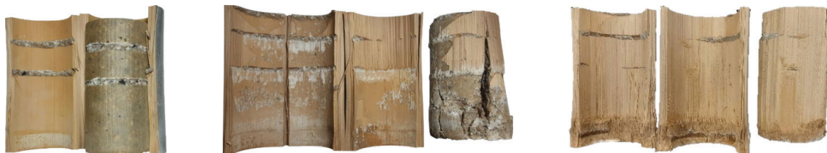
Figure 5: Specimen EP-71-9 with CBF < 10 % (left), specimen PU-71-5 with CBF ~ 50 % (middle) and specimen EP-251-4 with CBF ~ 100 % (right).
