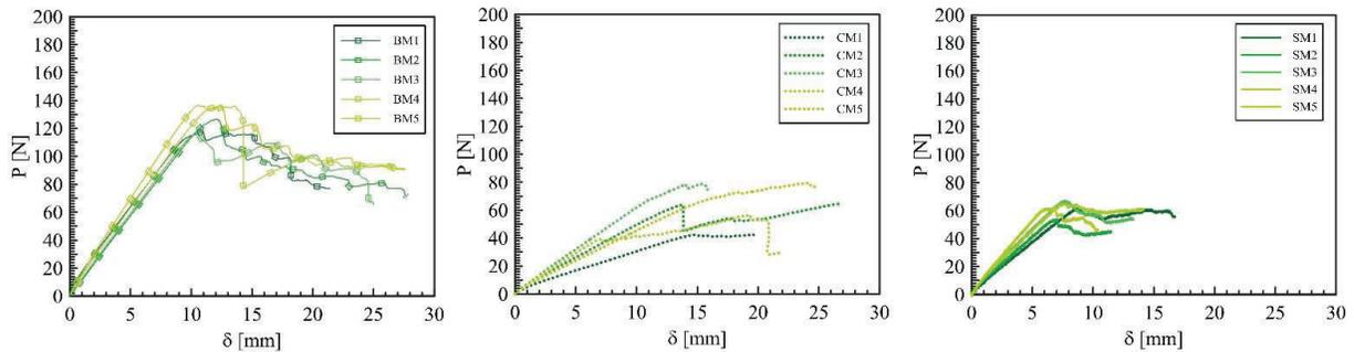
Figure 5. Load- Crosshead displacement for specimens with melamine adhesive: a) Beech; b) Chestnut; c) Spruce.
