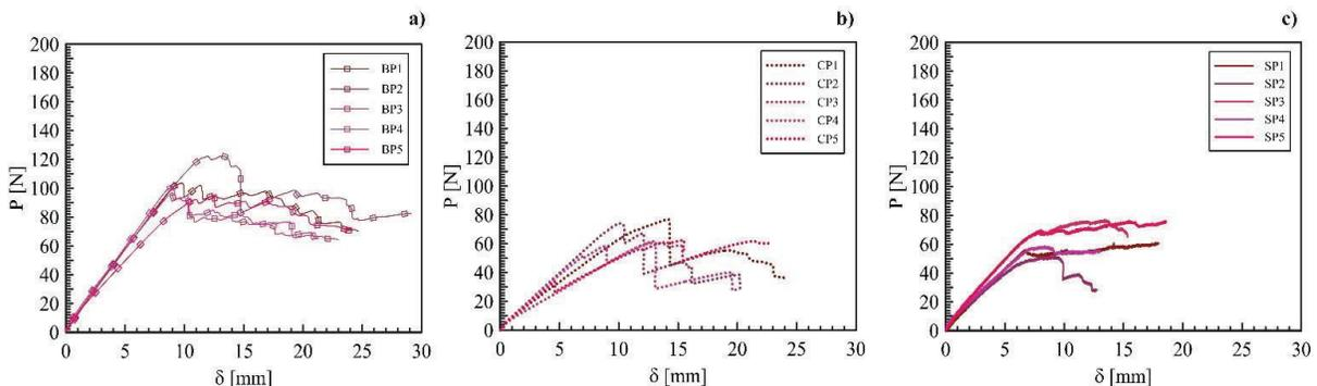
Figure 6. Load- Crosshead displacement for specimens with phenolic adhesive: a) Beech; b) Chestnut; c) Spruce.
