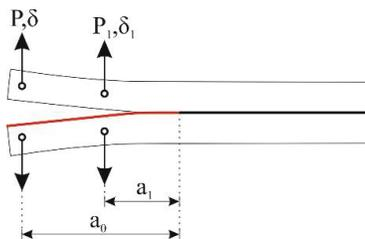
Figure 4. Determination of the root rotation correction factor  $\Delta$ .
