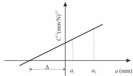
Figure 5. The definition of the  $\Delta$  parameter of the modified beam theory
