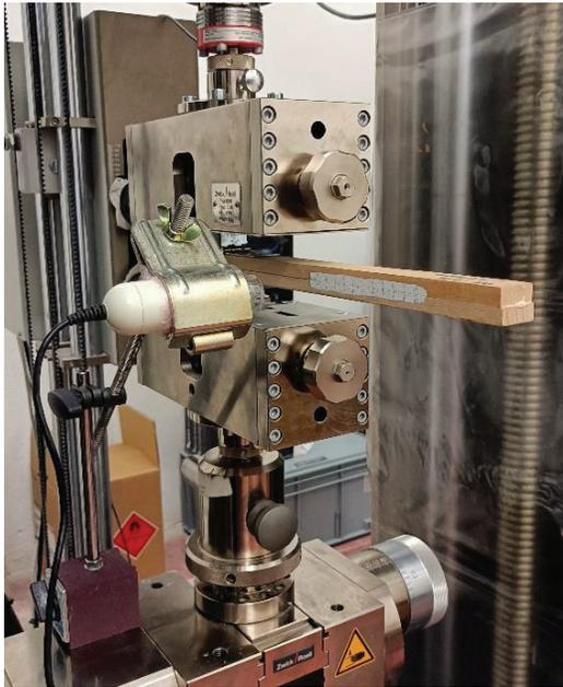
Figure 3. Setup including testing machine and optical microscope
