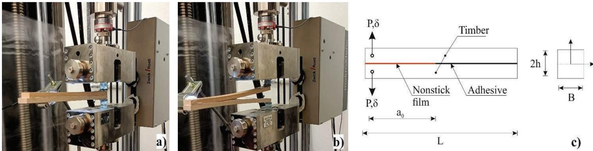
Figure 2. Specimen: a) starting point of DCB test, b) opening of DCB test, c) geometrical features
