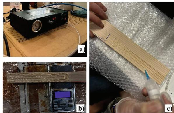
Figure 1. Specimen manufacturing: a) the glue spreading machine; b) the measuring of glue spreading rate, c) the glue line deposition
