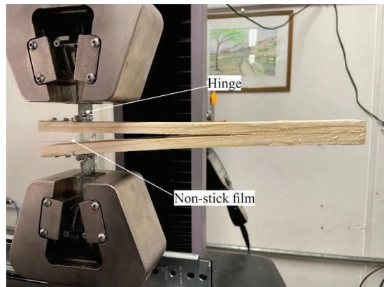
Figure 2. Specimen and hinges
