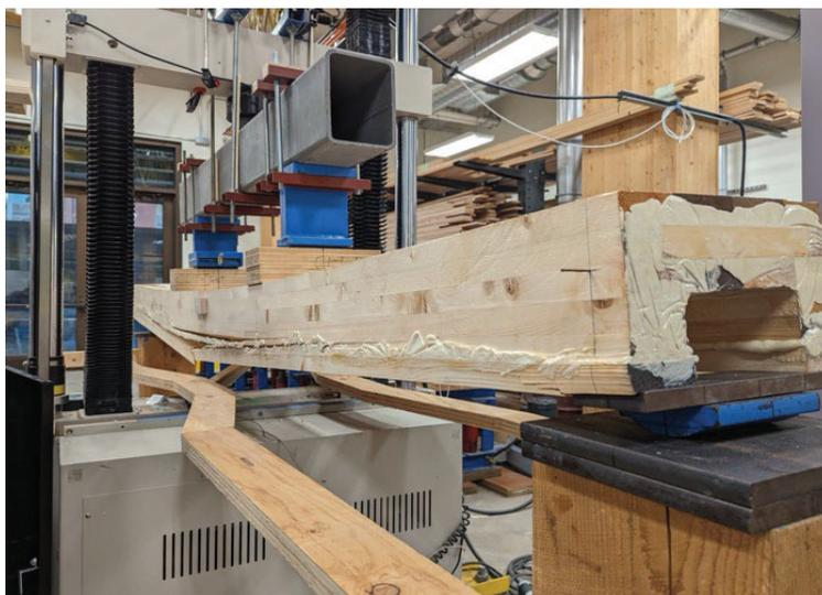
Figure 4 – Typical Failure Mechanism of 6 layer T-Beams
