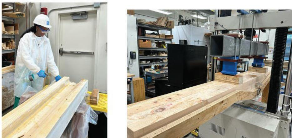
Figure 3 - Manufacturing and Testing of 6-layer CLT(Gs): primer sprayed for additional stem (left), flexural test configuration. (right)
