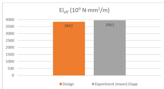
Figure 6 – Design vs Experimental Results for Bending Stiffness
