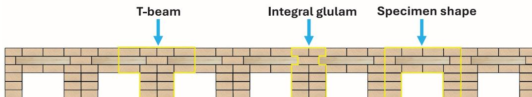
Figure 1 - Proposed T-Beam Floor System with Integral Glulam
