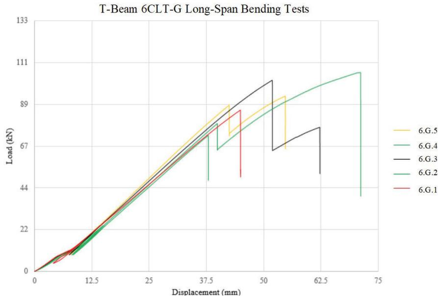
Figure 5– Load- Mid-span Displacement Graphs
