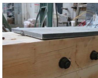
(b) Separation between steel plate and CLT
