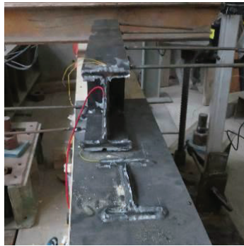
(f) Tensile fracture failure
