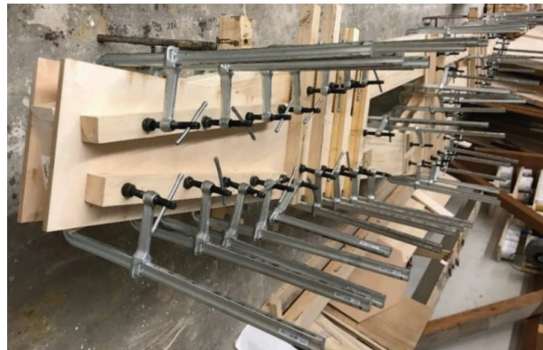
Figure 3. Assembly of a glued truss.
