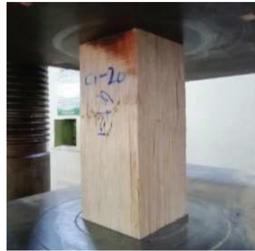
Figure 2. Compression tests specimens and loading apparatus.
