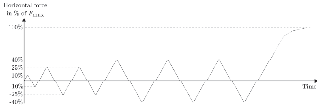
Figure 3: Loading protocol based on ISO 21581:2010, adapted for application in the experiments on the one-storey wall element with window openings. The protocol includes additional steps at 25% and 40% of the estimated maximum force F_{h,max,est} to account for serviceability criteria and stiffness evaluation under monotonic loading, unloading, and reloading conditions.
