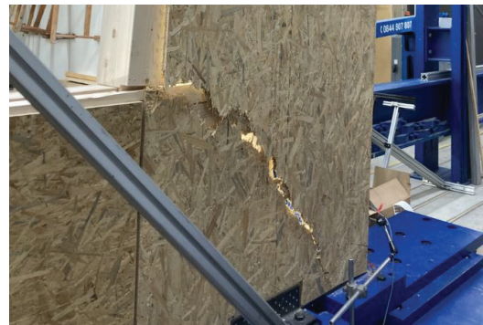
Figure 12: Brittle failure of the OSB/3 panel on the side opposite to the force application in Wall 2-3. Wall 2-4 exhibited a very similar failure pattern, but the OSB/3 panel failed on the side where the force was applied.
