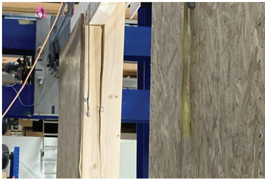
Figure 11: Brittle failure of the window stud on the side opposite to the force application in Wall 2-2, after reaching the maximum force. Wall 2-1 exhibited a very similar failure pattern.
