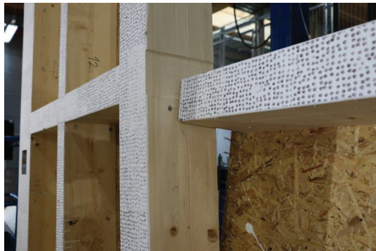
Figure 7: Out-of-plane displacements of the sill segment of Wall 1-1 and 1-4. The behaviour of Wall 1-1 and 1-4 was similar.
