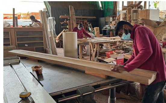
Figure 9. Left: Well Sphere – Transition from a straight base to a concave cornice, representing renewal and the resilience of nature. Right: Finishing of a 100 mm thick CNC-milled rain tree plank for Well Sphere columns. (Image courtesy of Tat Hin Timber)
