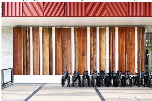
Figure 10. Rainbow Forum – A series of extra-large timber blocks hand-engraved into concave profiles using the Tree-to-Design approach, maximizing the potential of each harvested tree.
