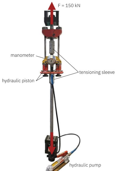
Figure 5: Tension rod with pretensioning system installed
