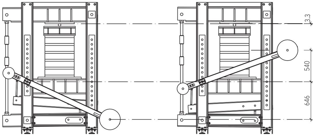
Figure 7: Kinematics of the levers: minimum (left) and maximum (right) positions of the first lever
