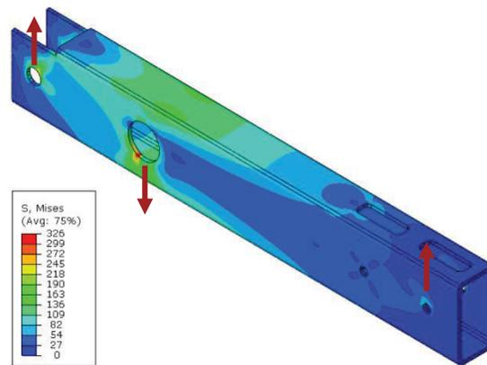
**Figure 4:** Finite Element Analysis of the third lever
