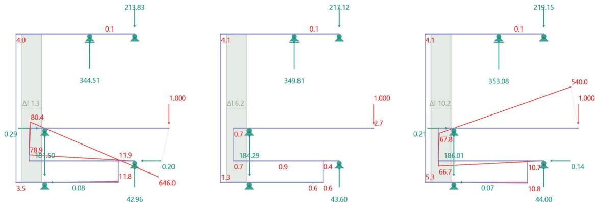
Figure 8: Calculations using 3rd order theory: Analysing the influence of the inclination of the levers
