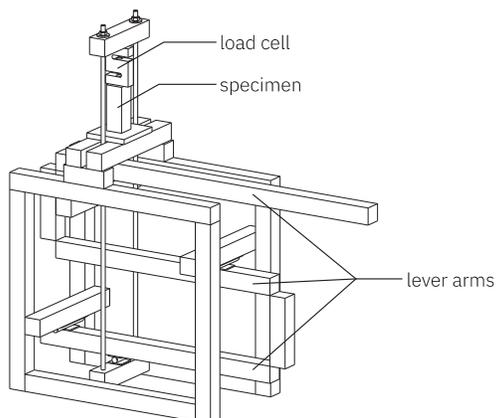
constant over time were specified as main objectives. To meet both requirements, the idea of a testing machine with several levers and deadweight seemed most suitable.
