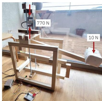
Figure 1: 3D-View of a prototype with three levers (left) and the actual prototype loaded with 10 N (right)
