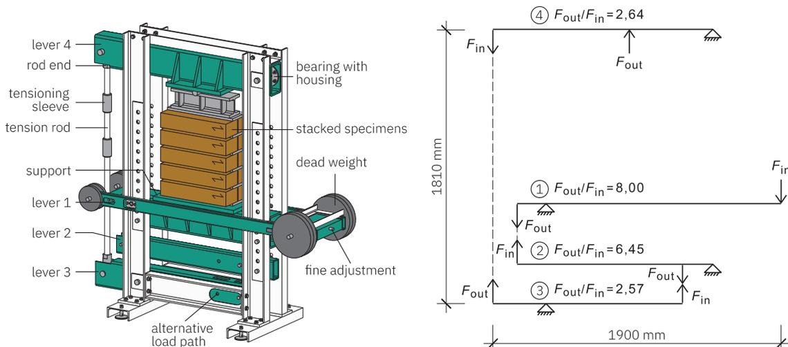
Figure 2: Final design of the developed creep testing machine (left) and the corresponding schematic sketch of the simplified mechanics (right)
