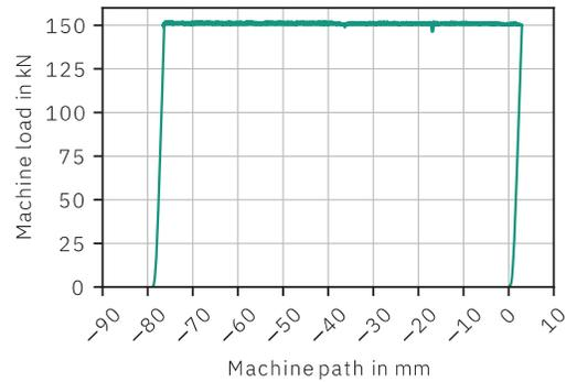
Figure 6: Load-displacement curve showing constant load while shortening
