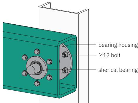
**Figure 3:** Connection of the levers to the frame using spherical bearings
