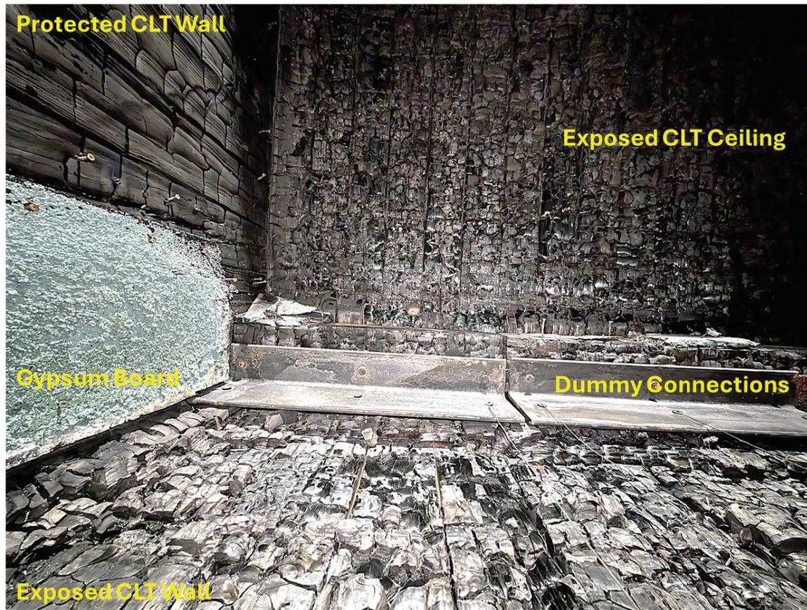
Figure 11: Charring patterns from different surfaces in Test 3.
