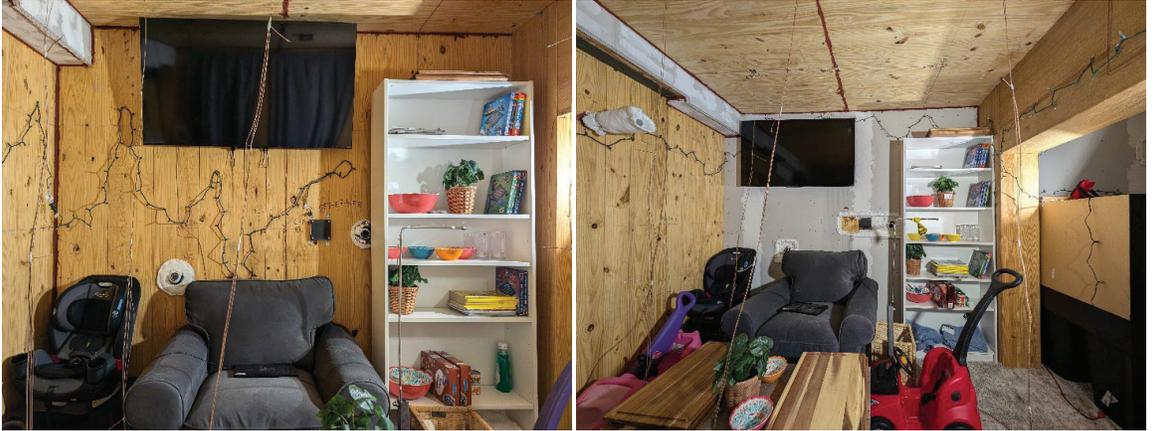
Figure 2: Varying amounts of exposed mass timber in back portion of Test #2 (left) and Test #3 (right) prior to testing.
