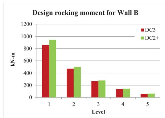
Figure 4. Design rocking moment for Wall B
