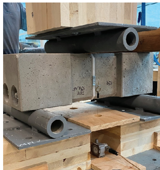
Figure 6 – Structural Testing with Steel Roller Supports
