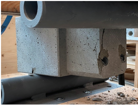
Figure 7 – TCN After Fracture of the Steel Tension Reinforcing Rods
