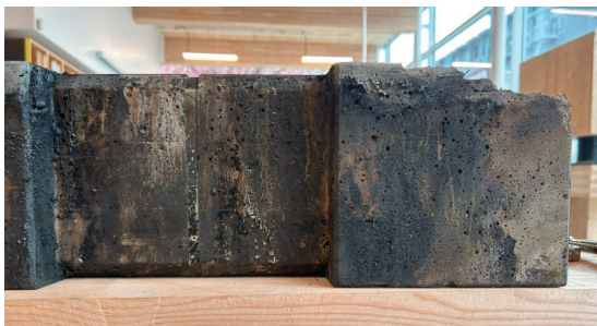
Figure 10 - TCN Following Post-Fire Structural Testing
