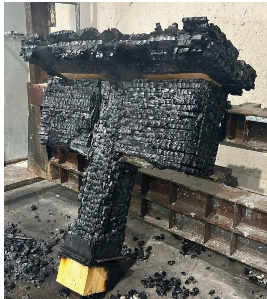
Figure 8 – TCN and Timber Assembly Post-Fire
