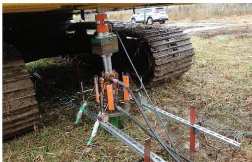
Figure 7 Photograph of the vertical loading test
