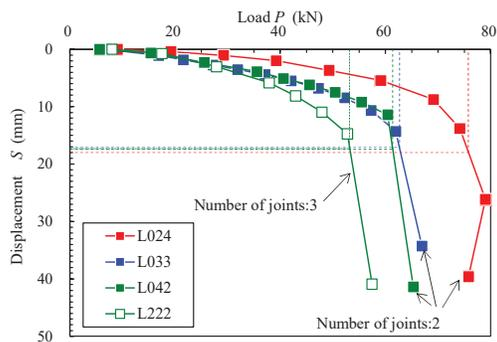
Figure 9 Relationship between the load and displacement in joined logs
