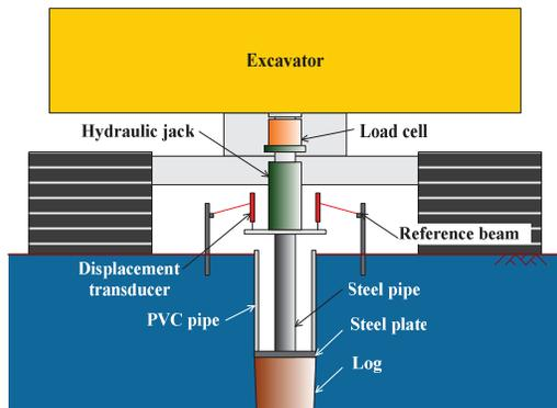
Figure 6 Schematic of the vertical loading test
