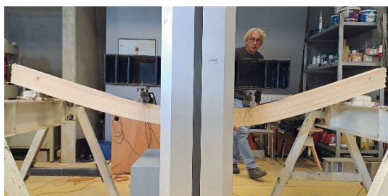
Figure 4: Characteristic failure of beam specimen with densified dowels with dowels installed alternately through the lamellas
