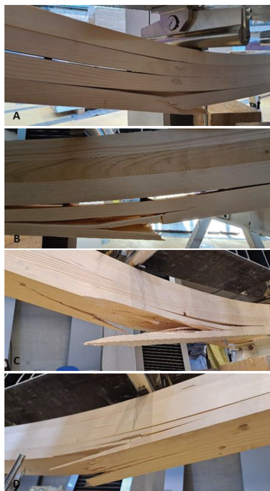
Figure 5: Characteristic failure of beam specimen with densified dowels installed alternately through the lamellas (A), welded dowels installed alternately through the lamellas (B), densified dowels installed vertically through the all lamellas (C) and densified dowels with dowels installed at a 45° angle through the all lamellas (D)
