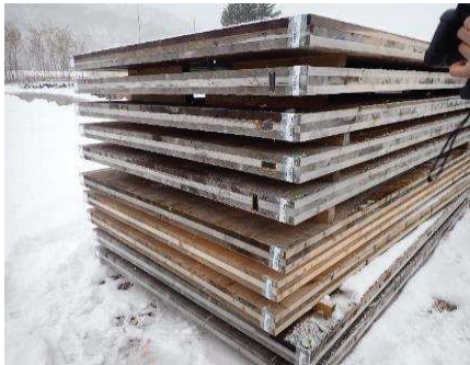
Fig.7: IC tag attached to CLT plates
