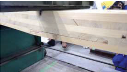
Fig.19: CLT specimen destruction
