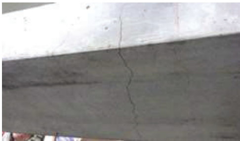
Fig.20: RC specimen destruction
