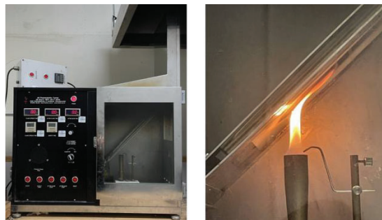
Figure 3. Test setup for flame-retardant evaluation using a 45 Degree Flammability Tester
