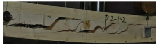
Figure 2. Rolling shear failure in a CLT specimen subjected to bending. Search: [2].
