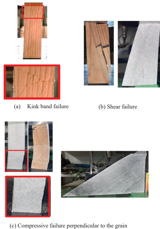
Figure 6. Failure modes of cedar specimens with or without side margin
