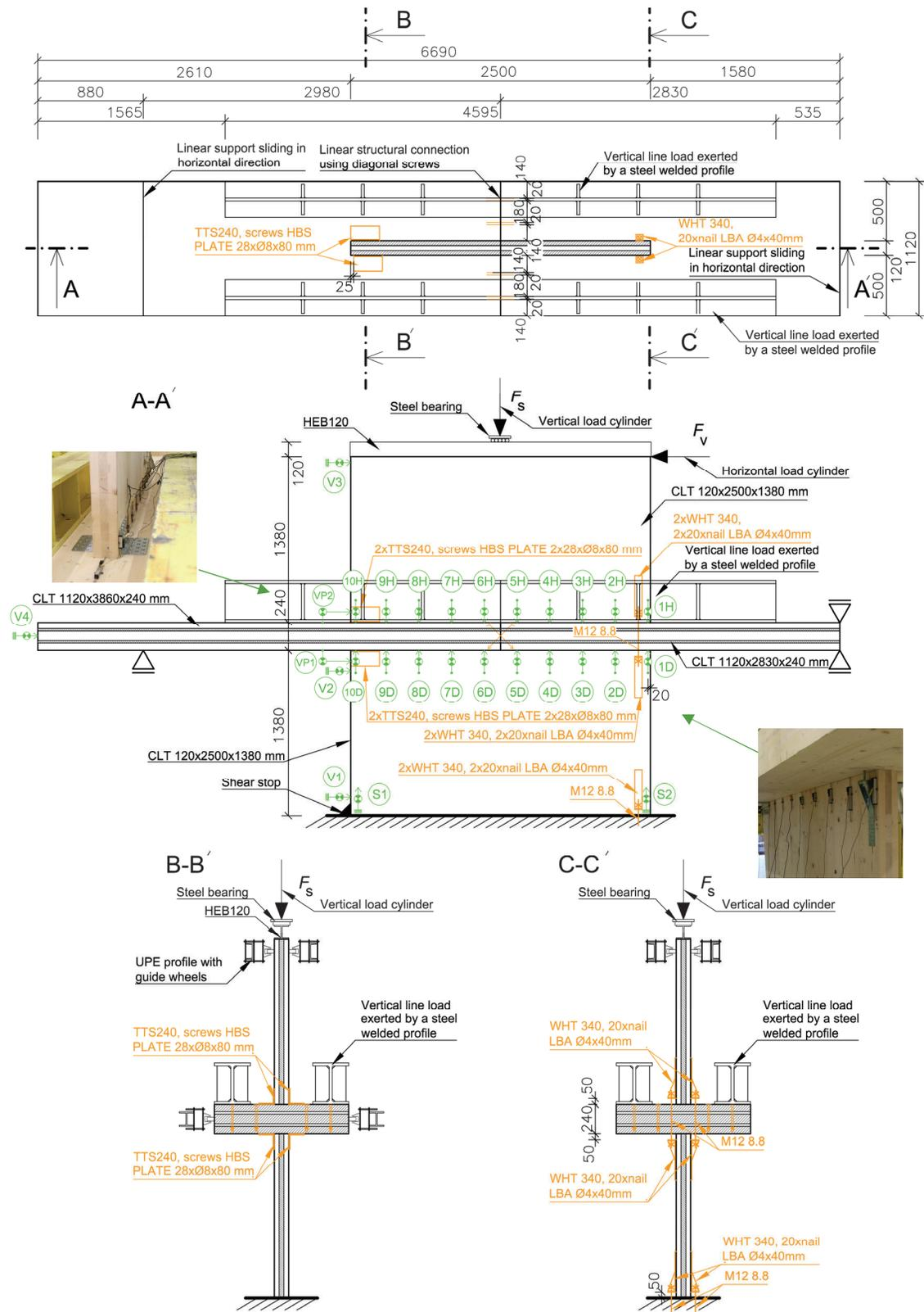
Figure 1. Wall to floor connection: scheme of the test set-up with display of anchoring and connecting elements (orange color) and sensor positions (green color).
