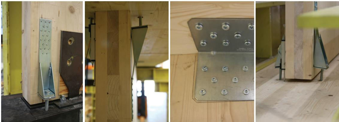
Figure 7. Observed failure of tension anchor and shear brackets in the connections of the full-scale test specimen.
