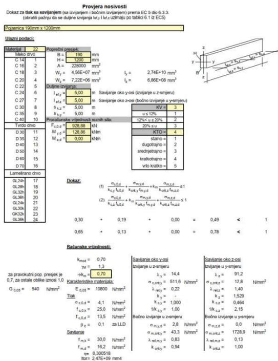
Figure 7. Dimensioning of the column wings at a height of 2.5 meters according to the ultimate limit state.
