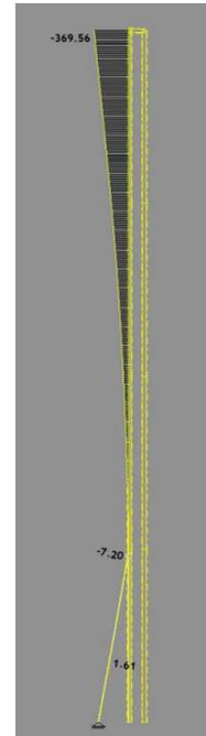
Figure 8. The maximum displacement of the column according to the serviceability limit state is 369.56 mm.
