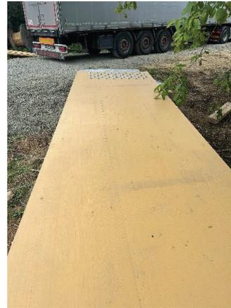
Figure 5. Glued laminated timber (GLT) wing elements of strength class GL30c.
