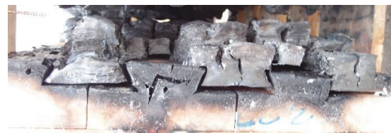
Figure 9. Remaining lamella layers and the dovetail structure of DMWBEs at the end of the test.
