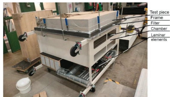
Figure 6. Air permeance test equipment.
