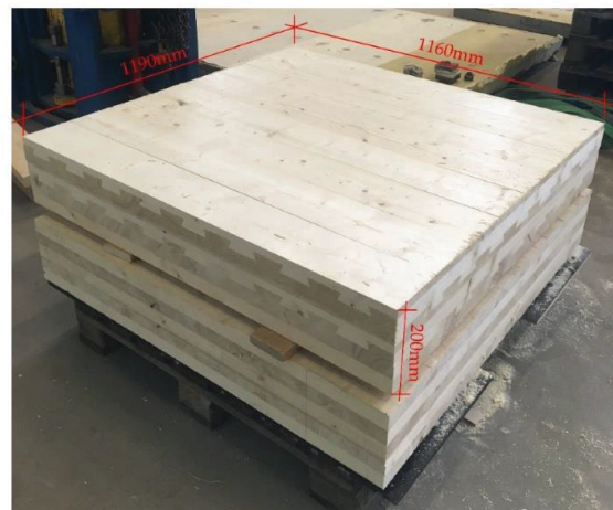
Figure 3. Test specimens: DMWBE (upper) and CLT (lower).
