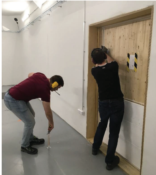
Figure 4. Mounting of sound insulation testing specimens.
