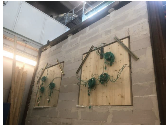
Figure 5. Mounting of fire performance testing specimens.
