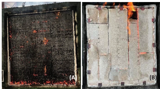
Figure 4. Specimens of CLT wall after fire test; (A) unclad CLT wall, (B) CLT wall clad by fireproof gypsum board.
