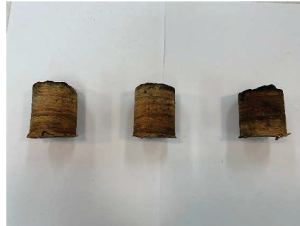
Figure 5. Specimens for measuring charring depth.
