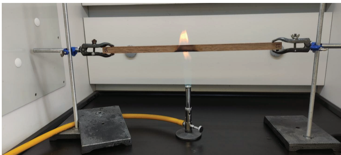
Figure 1. Flammability Test Setup According to Sotomayor Castellanos and Carrillo Gómez (2017).
