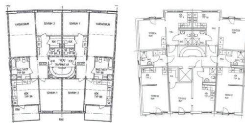
Figure 15: Floor plans showing a building section from the original donor building with two two-storey apartments (left), and the new student housing block with five apartments (right).
