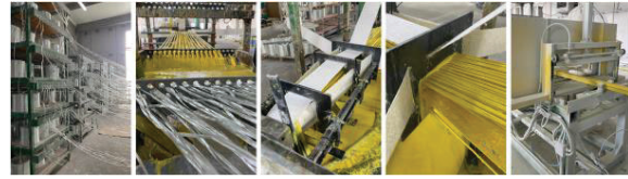
Figure 3: Right: Pultrusion process, roving racks, preforming guides, roving, surfacing mat – source [Italcomposites Doo]
