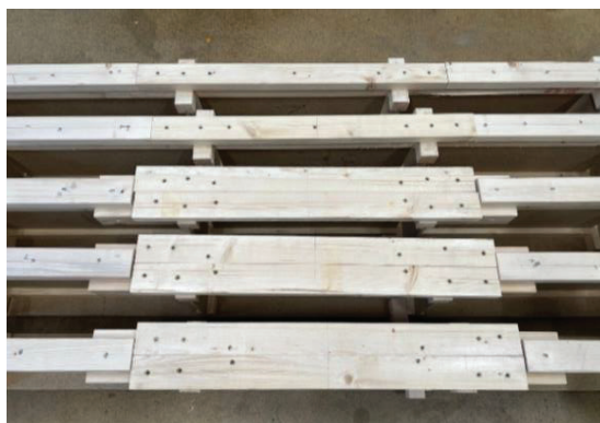
Figure 4: View of the elements from underneath with reassembly types 1, group A, (on the top) and type 2, group B, (at the bottom) after the first dis- and reassembly.
