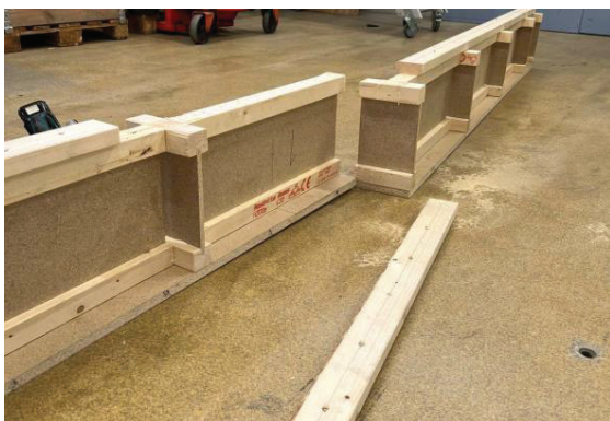
Figure 3: An example of a disassembled element after its first four-point bending test.
