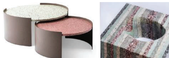
Figure 14: Panel and furniture obtained from the recycling of fibreglass and rigid expanded thermosets – source [Gees Recycling Srl]
