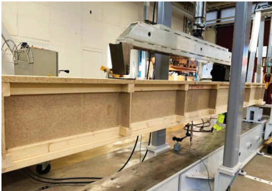
Figure 2: One of the flooring elements under the four-point bending test setup.
