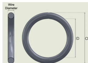
Figure 1. Chain mail ring dimensions indicating wire diameter, inner diameter (ID) and outer diameter (OD)
