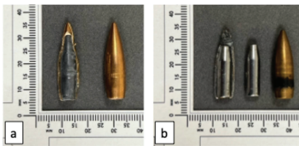
Figure 1. Projectiles used in this study (a) 7.62 × 51 mm LC and (b) 7.62 × 39 mm MSC
