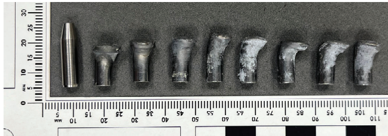
Figure 5. MSC cores from HAP #1 after the HVI test, cores are arranged in ascending shot order with the first one being the unused MSC core
