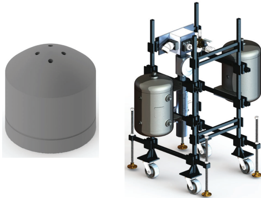
Figure 1. 3D-printed indenter modeled after backface deformation profile (left) and custom pneumatic impacting system for simulating BABT with live porcine specimens (right)
