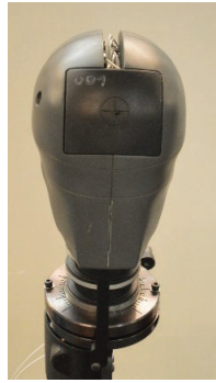
Figure 3.- Ballistic load sensing headform.
