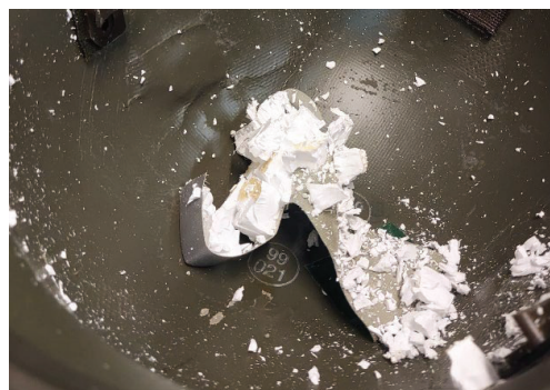
Figure 9. PMMA sample after the impact.
