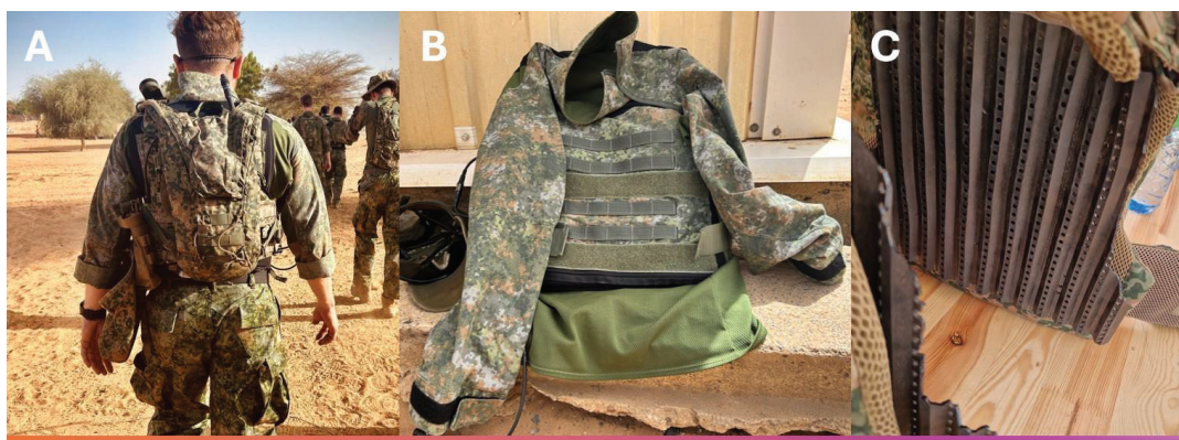
Figure 4. Example of active ventilated vest worn (A) and stand-alone (B) and the passive commercially available product on the inside of the ballistic configuration (C)
