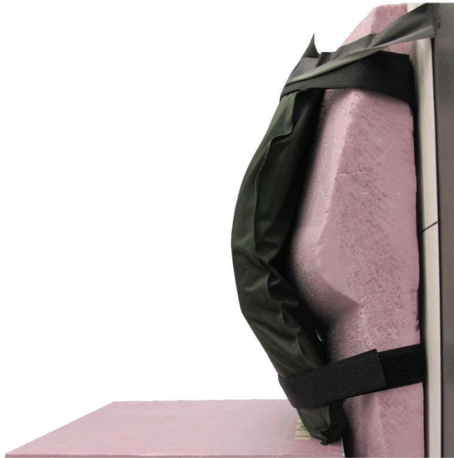
Figure 4 : NIJ 0101.07 C-5 Shape foam for radiography
