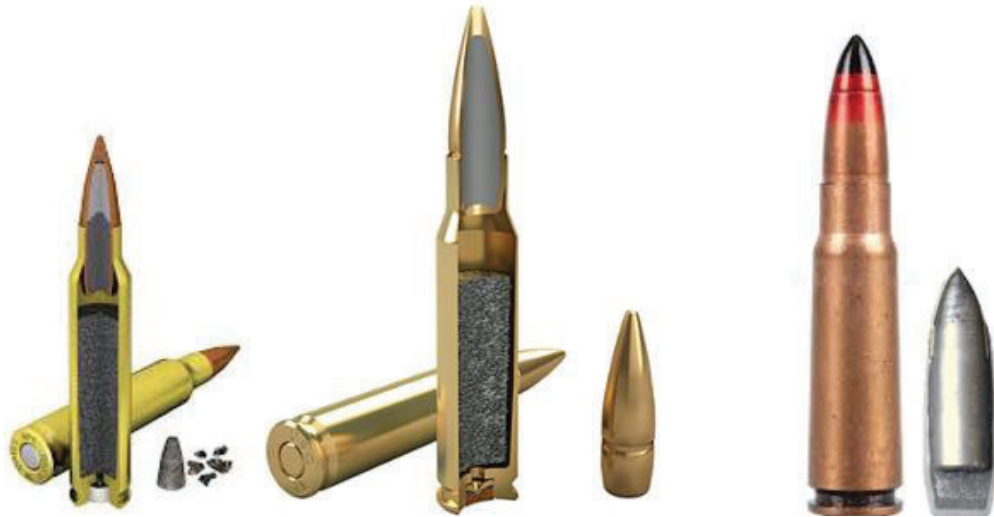
Figure 9 : 5.56mm Canadian C77 (Left), 7.62mm Canadian C21 (middle) and 7.62mm API-BZ Surrogate (Right).
