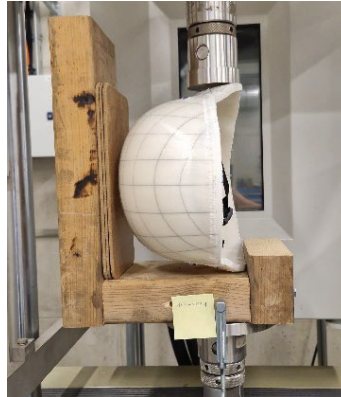
Figure 3: Side-to-side compression test setup with UHMWPE helmet shell sample.
