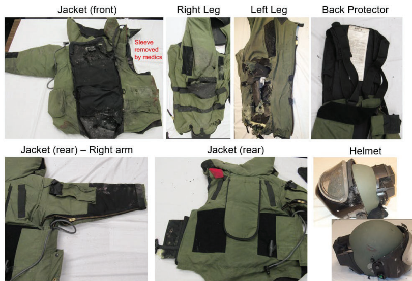
Figure 5. Photos of the bomb suit and helmet after the blast
