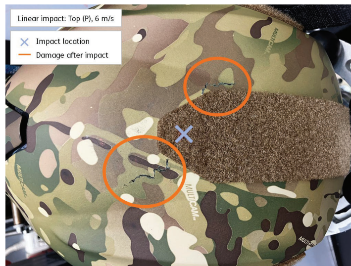
Figure 8. Damage to add-on shell after linear impact at 6 m/s at top location.
