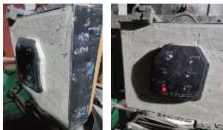
Figure 3: BFS measurement setup with P1 plastina.
