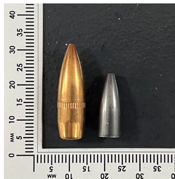
Figure 3. 7.62 mm HSC projectile and its hardened steel core
