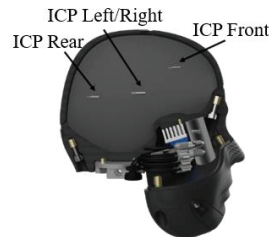
Figure 2. CAD Rendering of WBATD Headform showing the ICP sensor locations. The ICP Left and ICP Right sensors are symmetrical with respect to the mid-sagittal plane
