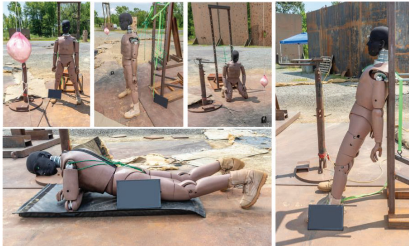
Figure 8. Various orientations, postures and PPE conditions (not shown) were tested. The WBATD is free-standing prior to the shot. The NIJ Integrity Test Stand prevents it from falling to the steel pad.
