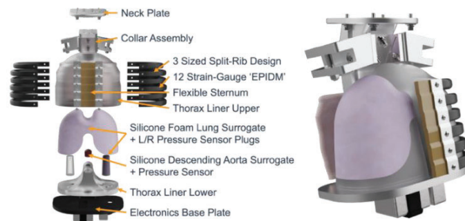
Figure 3. Exploded WBATD torso components (left) and cutaway view of the torso (right)
