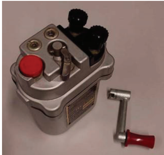
Figure 2. Blast machine used in military applications
