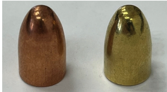
Figure 1. Sample projectiles taken from lots used in this evaluation of the copper (left), and brass (right) variants of the Remington 9mm Luger 124 grain FMJ ammunition
