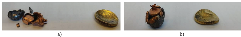
Figure 7. a) and b) Example of a 50 cents euro coin and .44 Magnum JHP ammunition after an impact (full vest penetration)
