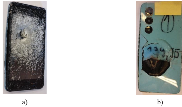
Figure 10. Example of a full penetrating smartphone test (polyethylene vest and the .44 Magnum projectile): a) front side; b) back side
