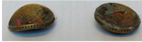
Figure 4. 50 cents euro coin after an impact (full vest perforation)
