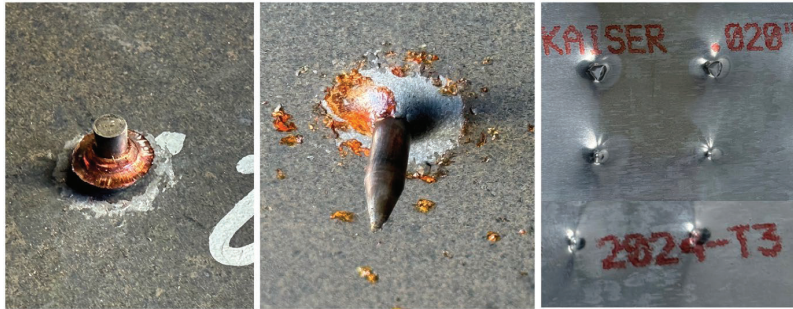
Figure 1: Embedded projectile in an armour plate: front (left), rear (centre), and witness sheet (right).
