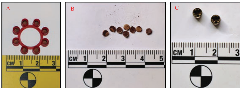
Figure 4. A) Cap gun ring. B) 8 recovered caps. C) 2 assembled cap gun activated primers.
