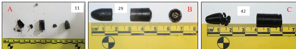
Figure 11. Numbers relate to shot reference in Table 1. A) Misfire, Suffered catastrophic casing failure upon strike from firing pin. B) Successfully fired at steel sheet, projectile recovered, case fracture at primer pocket. C) Successfully fired at steel sheet, projectile recovered showing impact damage.
