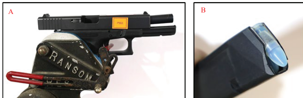
Figure 9. A) Glock 17 mounted in Ransom Rest. B) Glock 17 Magazine loaded with three rounds of 3D printed ammunition.
